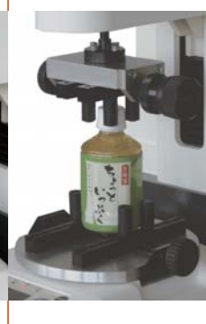
Supports HACCP and GMP. Opening/fitting force of caps
